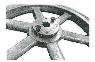
Insert the bushing gently into the sheave and thread the bolts by hand through the NON-THREADED holes of the Bushing. Do not tighten these bolts yet
